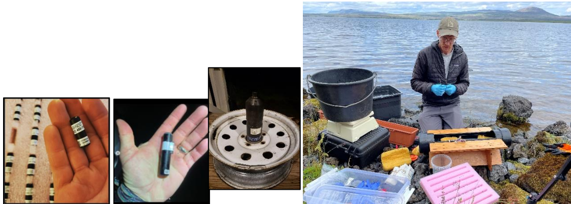
Pictures of equipment used in acoustic telemetry study; v9 transmitter, v16 transmitter, VRT2x acoustic receiver and example of on-site surgery station.
